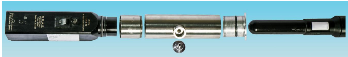
Figure 108. Split view of a G.R.A.S. 42AC pistonphone calibrator with an M36 hydrophone.
