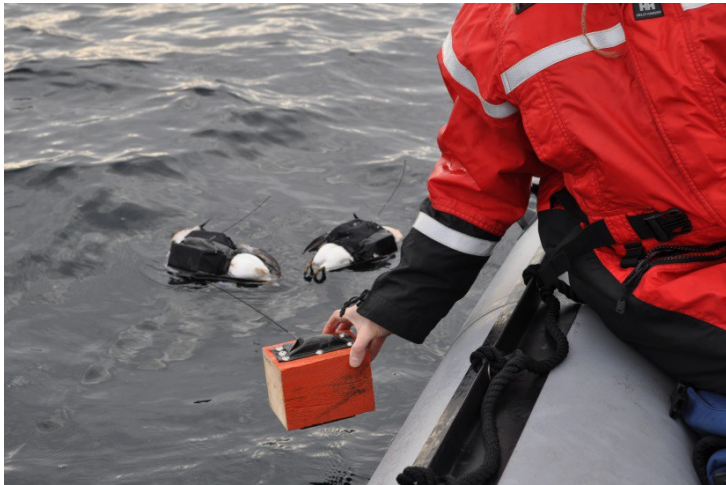
Figure A-2. Drift block and bird carcass deployments outside Witless Bay, Newfoundland and Labrador, for Phase I proof of concept.
