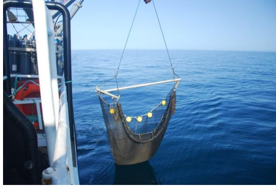
Figure 21 Deployment of the 3 m benthic beam trawl (BBT), the primary gear for sampling epibenthic invertebrates.
