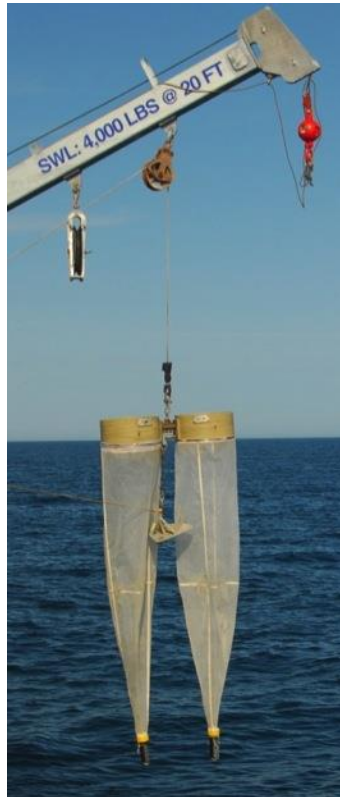
Figure 24 Bongo net for oblique sampling of plankton and larval fish.
