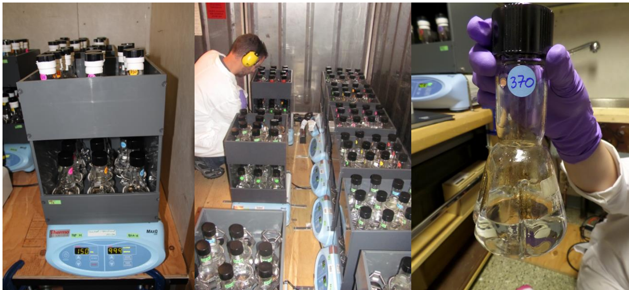
Figure 1-1: Photos showing the setup of microcosms in the refrigerated reefer. The copper colored disk next to label 370 (right side photo) is the oxygen sensor.
