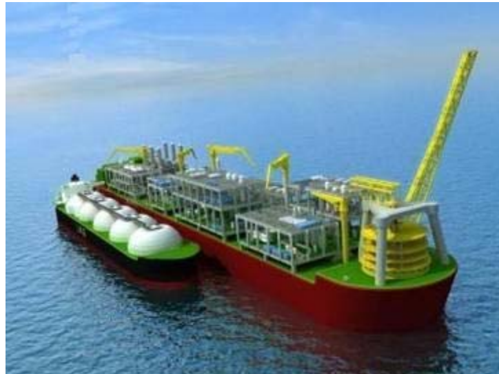
Figure 4-2: Sample Floating LNG Plant (Ref. /27/)
