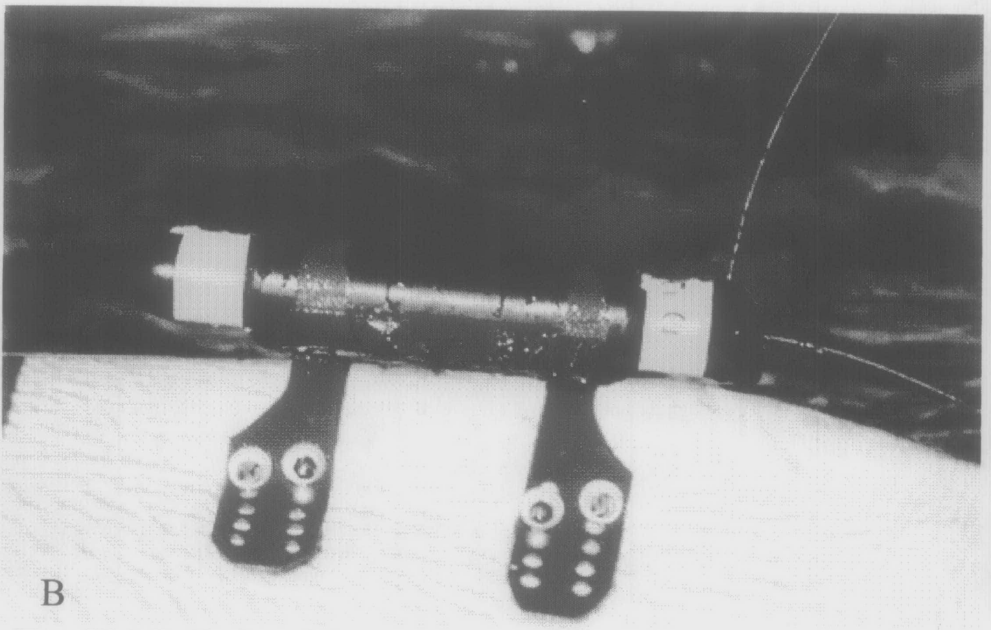
Figure 2.3: A- Double-tube tag design and attachment used in 1993 and some of the 1995 tags; B- Single-tube tag design and attachment used on 12 of the 1995 tags.
