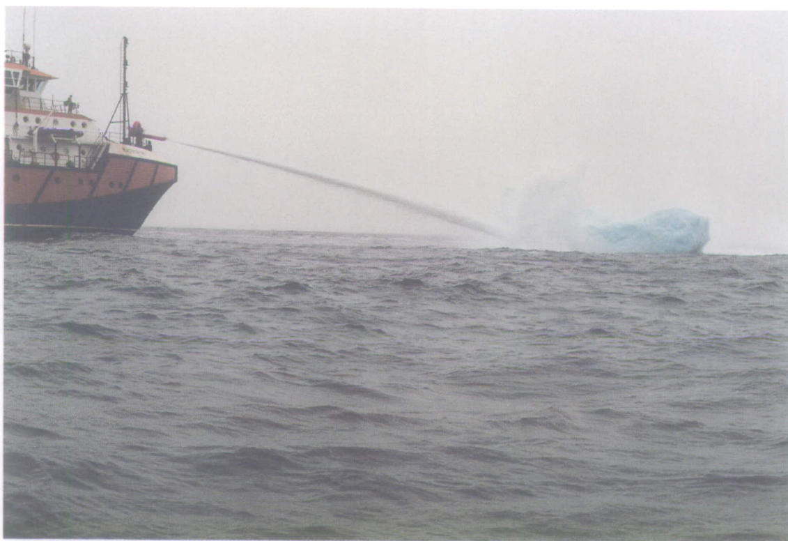
Figure 15. Water cannon operations with water jet striking the sail just at the water line.
