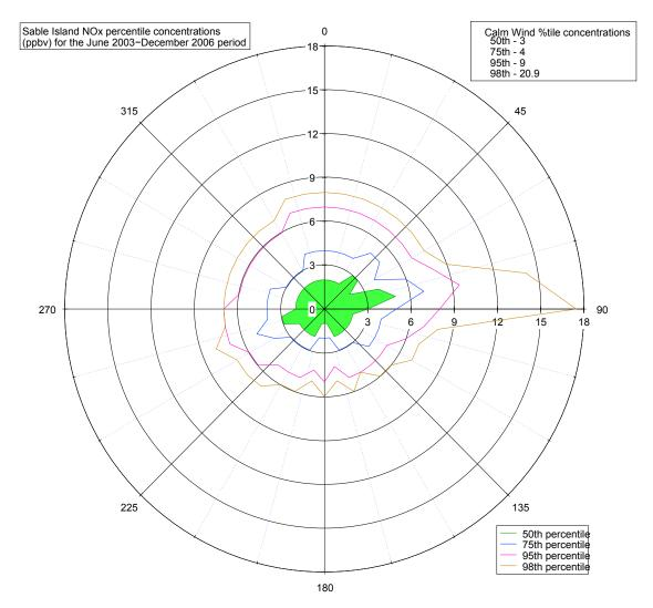
direction of 70–90 degrees, which coincides with the location of the diesel generator on Sable Island as well as the Venture offshore platform and its diesel generators.
