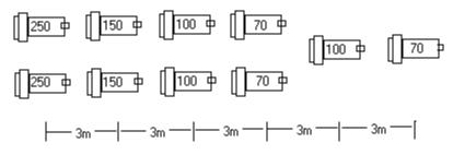
Figure 1.4: Airgun array layout.
