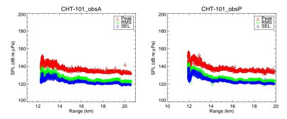
Figure 1.13: Peak, RMS, and sound exposure level measurements versus range obtained at OBS-A at 63-m depth (left) and OBS-P at 70-m depth (right). Measurements were taken during seismic Line CHT-101-01 with a heading of 89 degrees on the closest approach to the control site on Dec. 15, 2003.
