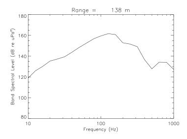
Figure 1.11: Third-octave band spectral levels as a function of frequency for an airgun event received at CPA (138 m) to OBS-P on Dec. 20, 2003, while the Admiral acquired data along line CHT-108-08.
