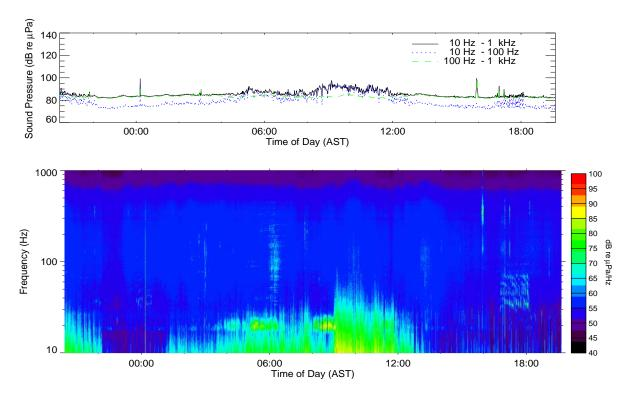
Figure 1.16: Ambient noise recording for 22 hours starting at 20:25:30 AST on December18, 2003.
