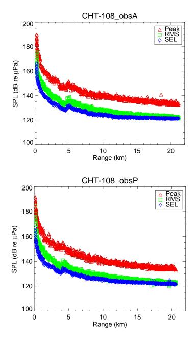
Figure 1.9: Peak, RMS, and sound exposure level measurements versus range obtained at OBS-A at 63-m depth (top panels) and OBS-P at 70- m depth (bottom panels) at the crab test site. Measurements were taken during seismic Line CHT-108-08 with a heading of 269 degrees through the test site on Dec. 20, 2003.
