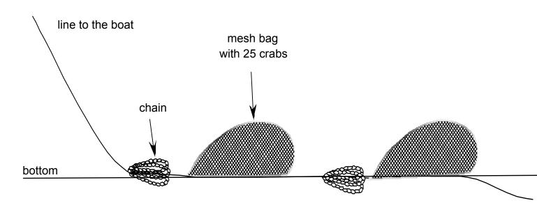
Figure 2.2: Schematic presentation of dragging bags containing female snow crabs.
