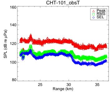
Figure 1.12: Peak, RMS, and sound exposure level measurements versus range obtained at OBS-T at 85-m depth at the control site. Measurements were taken during seismic Line CHT-101-01 with a heading of 89 degrees on the closest approach to the control site on Dec. 15, 2003.
