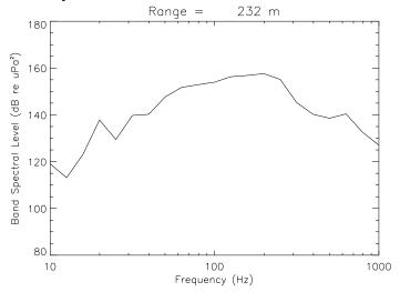
Figure 1.10: Third-octave band spectral levels as a function of frequency for an airgun event received at the CPA (232 m) to OBS-A on Dec. 20, 2003 while the Admiral acquired data along line CHT-108-08.
