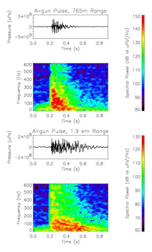
Figure 1.8: Plots of the pressure and spectral power for an individual airgun pulse measured on Dec. 20, 2003 at 1900-m range (right) and 765-m range (left). Admiral was acquiring data along line CHT-109-09 during these measurements.
