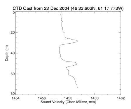
Figure 1.3: Sound speed profile from CTD cast performed on December 23, 2003, at location lat. 46°33.603'N, long. 61°17.773'W.
