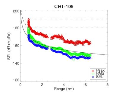
Figure 1.7: Peak, RMS, and sound exposure level measurements versus range at 34-m depth during seismic Line CHT-109-09 on Dec. 20, 2003. Solid black line indicates a fit of the transmission loss equations to the data beyond 1-km range ("endfire" levels). Dotted black line indicates a fit of the transmission loss equations to the data within 1 km range ("broadside" levels).
