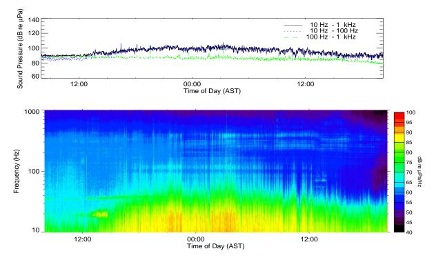
Figure 1.14: Ambient noise recording for 36 hours starting at 08:00:00 AST on December 13, 2003.
