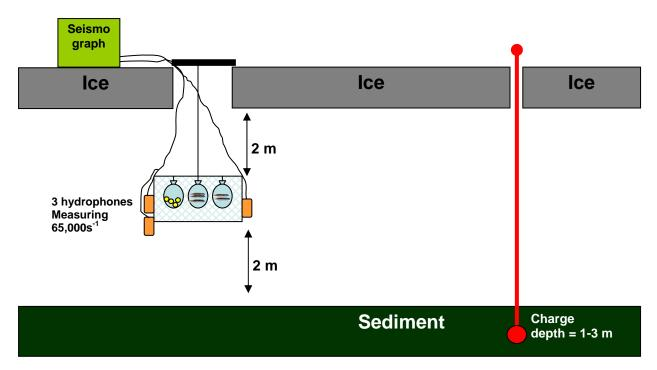
Figure 1: Schematic of IPC exposures.
