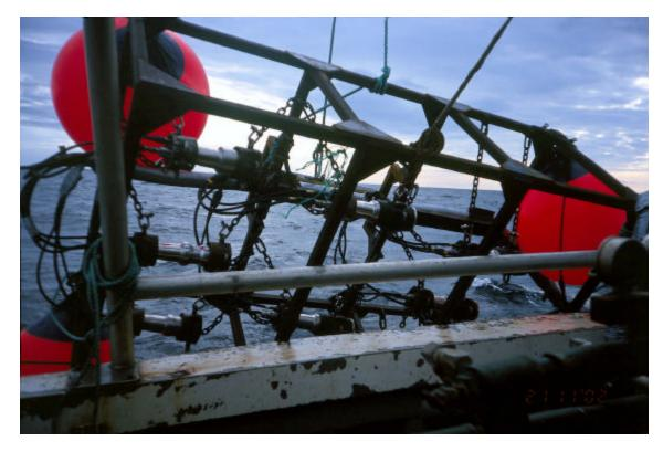
Figure 3. 200-in<sup>3</sup> seven-air gun array in frame.
