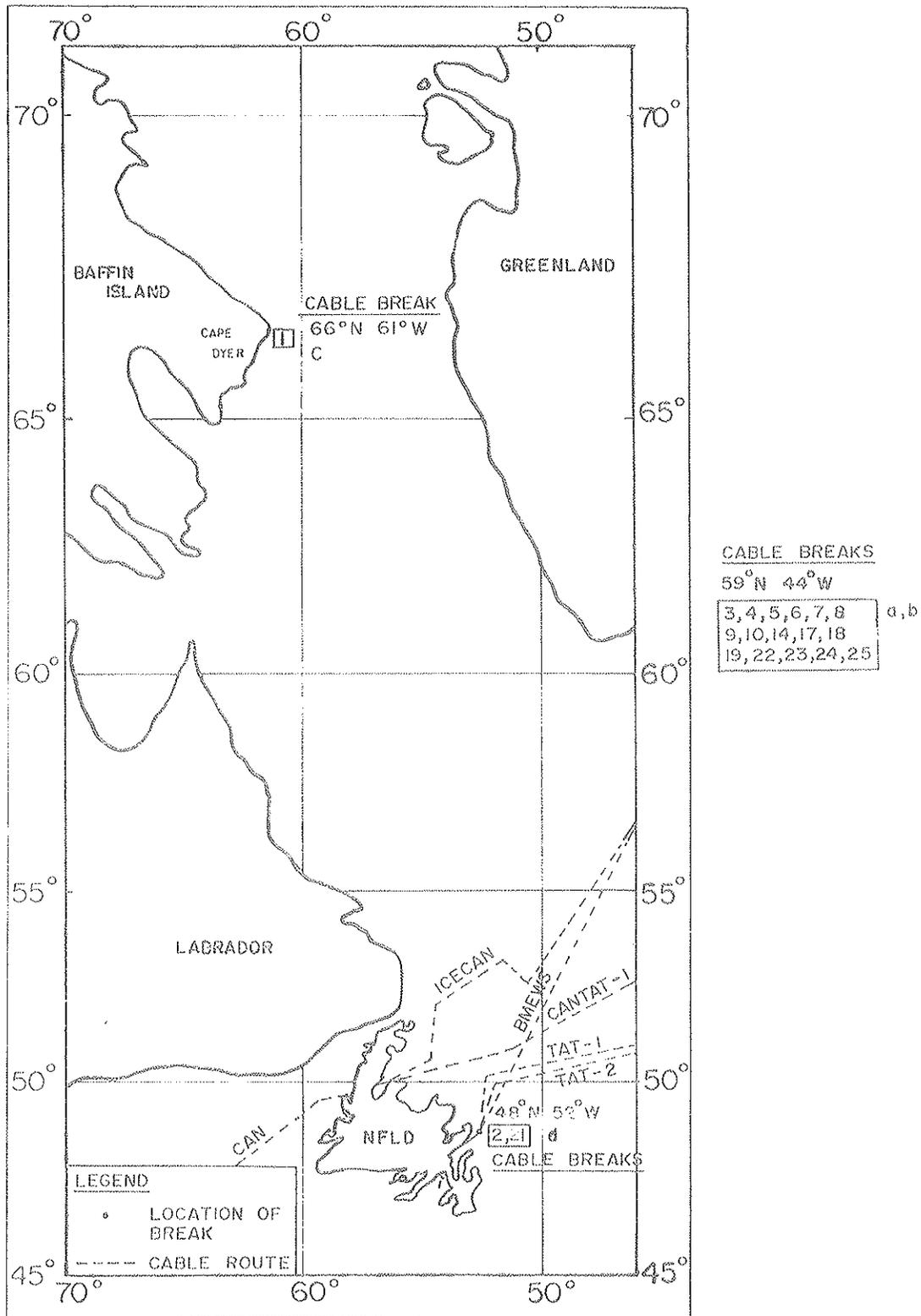
Fig. 7 Submarine cable routes and breaks caused by iceberg impact off Canada's East Coast
